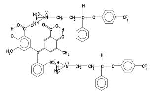
This formula conforms the spectrophotometric results (Job's and spectrophotometric titration methods) and the molar ratio ECR:FXT = 1:2.
